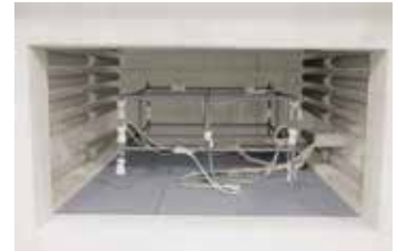
Measurement set-up in an annealing furnace
